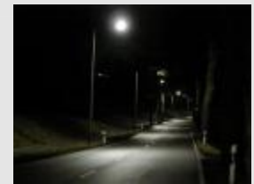
30 Watt LED-lamps replacing 125 Watt HQL-lamps ( federal road in Vogtland)
